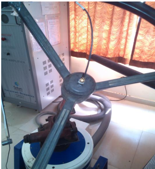
Figure 11: location of accelerometer when steering system is mounted on shaker machine
