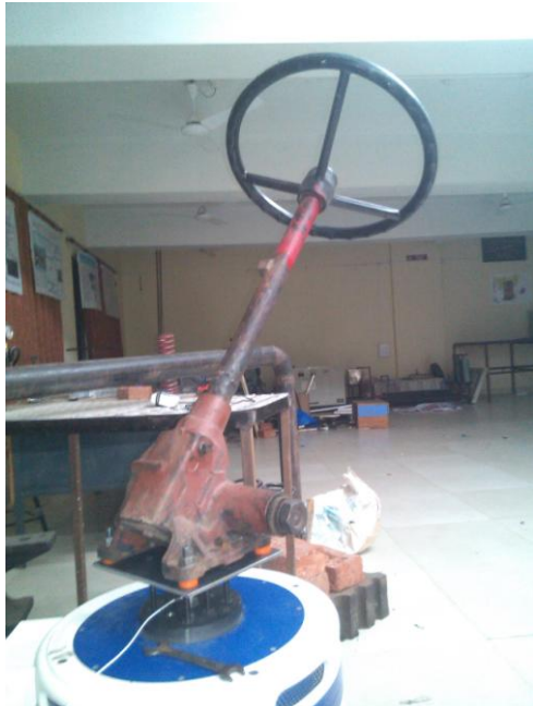
Figure 10: Experimental setup on shaker
