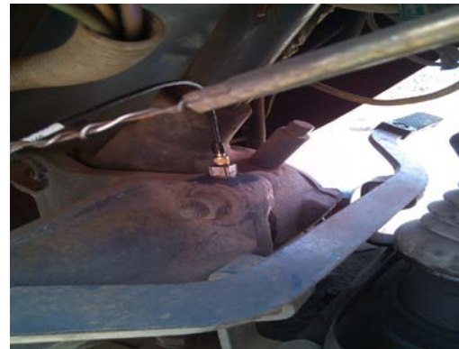
Figure 4 Accelerometer mounting at steering box
