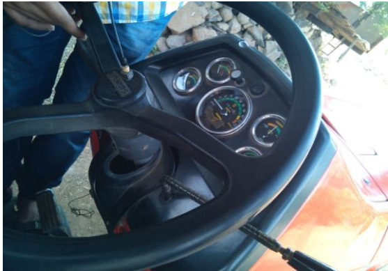
Figure 3: Accelerometer mounting at steering wheel
