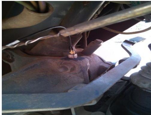
Figure 4: Accelerometer mounting at steering box
