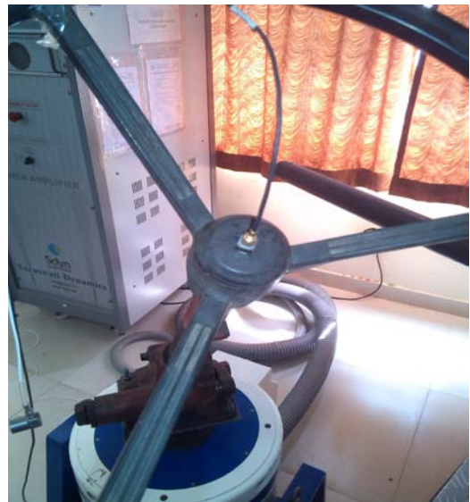
Figure 11: location of accelerometer when steering system is mounted on shaker machine
