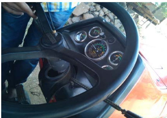
Figure 3. Accelerometer mounting at steering wheel
