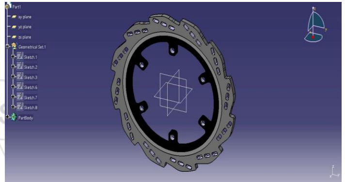
Figure 5: Petal disc brake rotor model in CATIA
