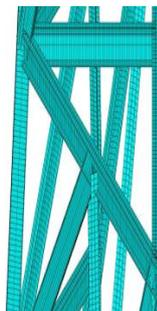
Figure 3: 3D Model of Tower with I Section
