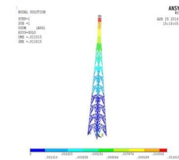
Figure 9: Displacement Diagram of Circular Section (Seismic Analysis)
