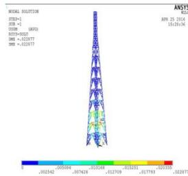
Figure 7: Displacement Diagram of I section (Seismic Analysis)
