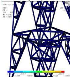
Figure 8: Stress Distribution Diagram of I section (Seismic Analysis)
