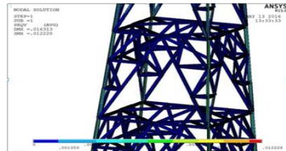
Figure 12: Stress Distribution Diagram of Channel Section (Seismic Analysis)
