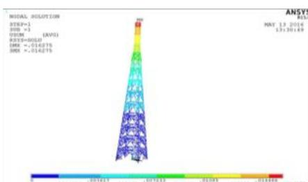
Figure 11: Displacement Diagram of Channel Section (Seismic Analysis)
