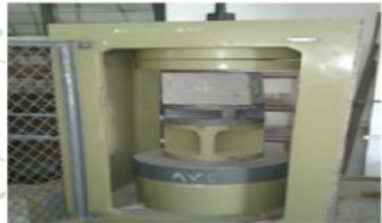
Figure 1: Concrete cube 150x150x150 testing
