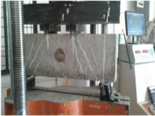
Figure 4: Bending Test on Various Beam
