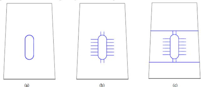
**Figure 2: Type 1, Type 2, Type 3 Stiffeners**
