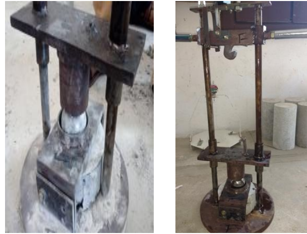
Figure 2: Drop weight test set up
