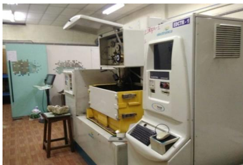
Figure 2(a): Electronica Ultracut S2 Wire-EDM
