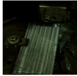
Figure 2(b): EN31 during wire EDM process
