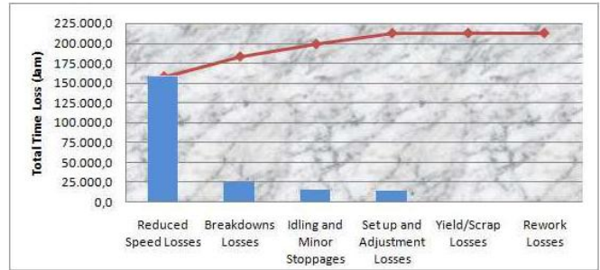
Figure 1: Pareto chart of the percentages of the Six Big Losses factors on the Weaving machine
