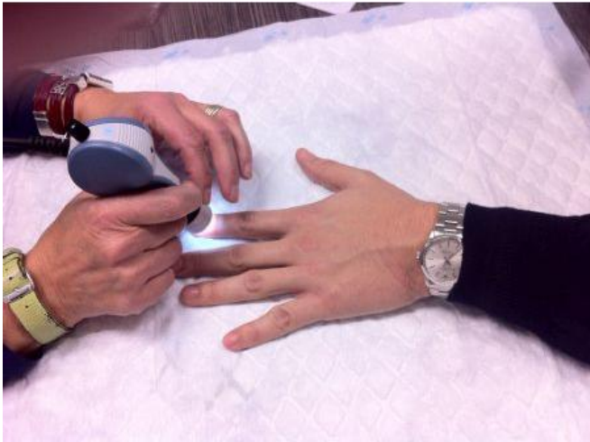
Figure 8: A prototype demonstrating a portable microscope placed manually on the patient's fingertip to take videos of microcirculation in very peripheral capillaries (Credit: Research Laboratory of Electronics/MIT)
