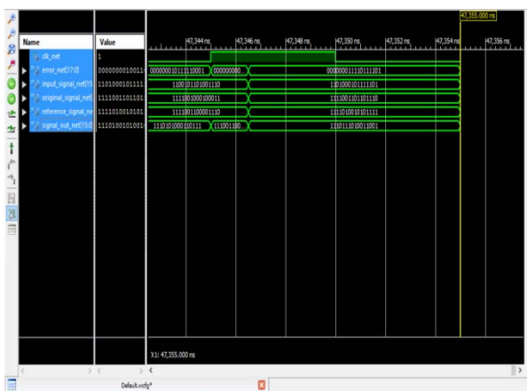
Figure 7: VHDL simulation system for LMS filter
