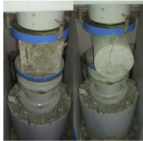
Figure 4: Compressive and tensile test of cube and cylinder
