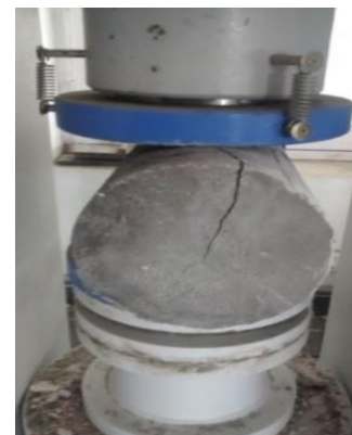
Figure 7: Tensile test on cylinders
