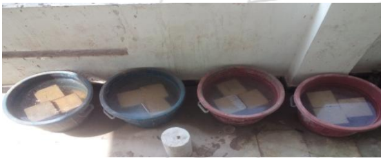
Figure 4(b): showing cubes in curing
