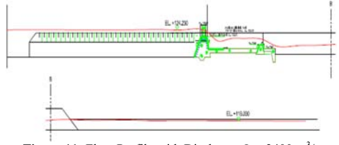
Figure 11: Flow Profile with Discharge Q = 2400 m 3 /s
