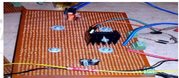
Figure 11: Hardware Prototype of Boost Chopper and Sensing Circuit
