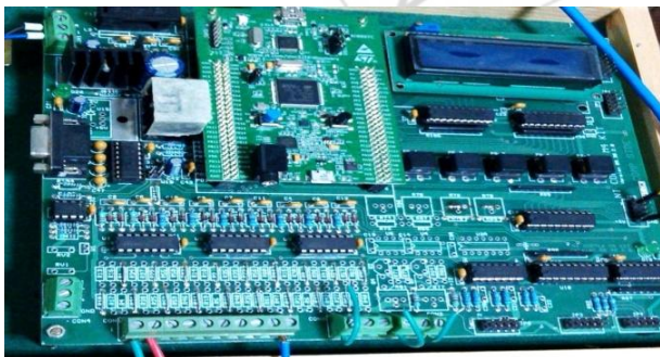
Figure 12: STM-32 Microcontroller Kit
