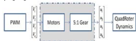
Figure 2: Motor and gear control
