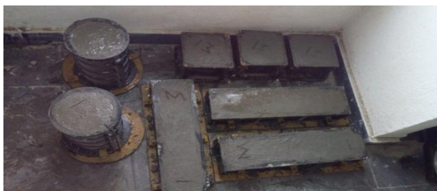
Figure 2: casting cubes, beams and cylinders
