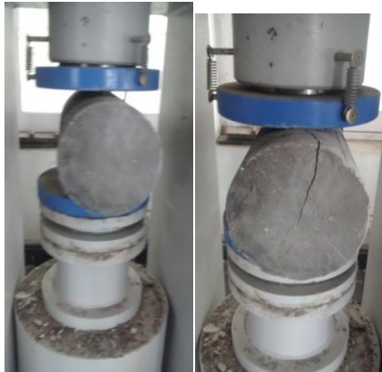
Figure 4: Tensile test on cylinders
