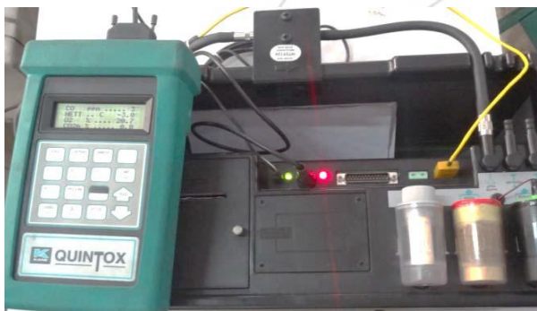
Figure 9: Flue Gas Analyzer
