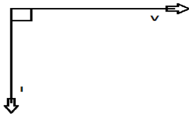
Figure 3: Current & Voltage 90° shifted
