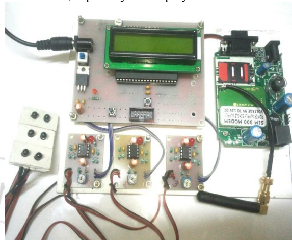
Figure 7: Hardware For Data Acquisition System to determine Prakriti of Person.
