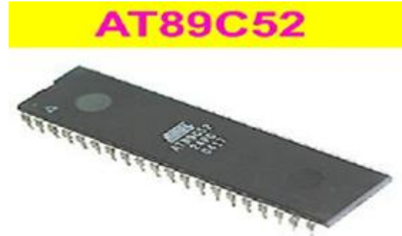
Figure 7: AT89C52 pictorial diagram
