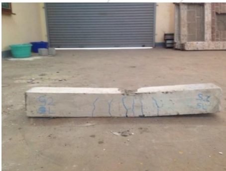
Figure 18: Crack pattern of S2SL specimen
