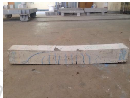
Figure 21: Crack pattern of S6DL specimen
