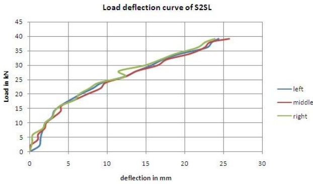
Figure 11: Load deflection curve of S2SL
