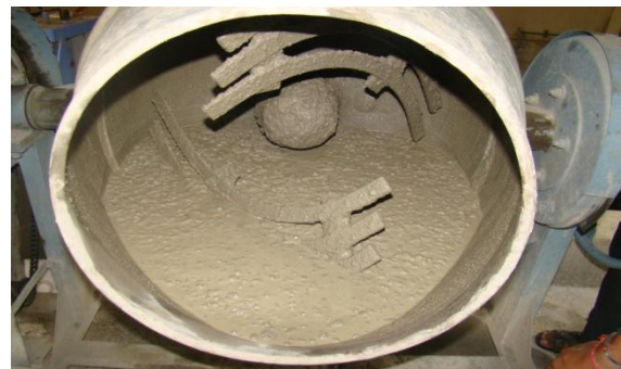
Figure 4: Self compacting concrete mix in the electronic drum mixture
