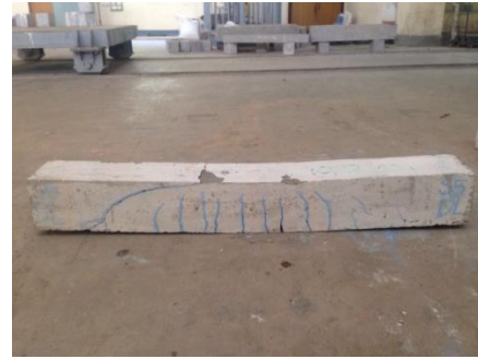
Figure 21: Crack pattern of S5DL specimen
