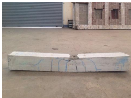
Figure 20: Crack pattern of S4SL specimen
