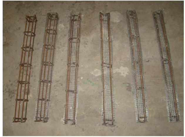
Figure 2: Reinforcement of beam specimens
