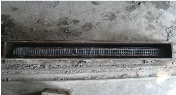
Figure 5: The casting mould and the reinforcement of the specimen
