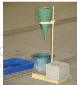
Figure 3: Marsh cone test for finding super plasticizer dosage
