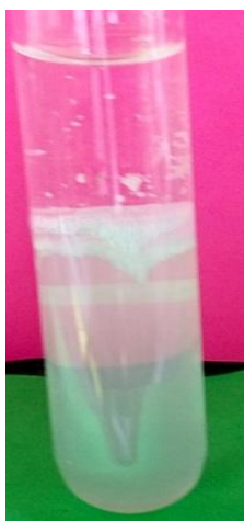
Figure 1: Growth of COM Crystals in Gel Medium.
