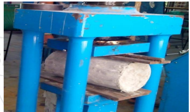
Figure 4.7: Split tensile strength test
