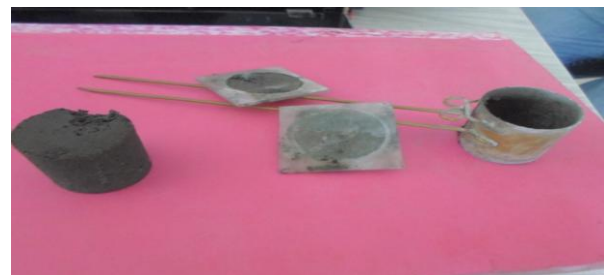
Figure 3.8: Le Chatelier Apparatus
