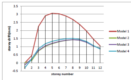
Figure 3.4: Storey drift in mm for load combination 21(D.L+LL+EQZ) along Z-axis for all models
