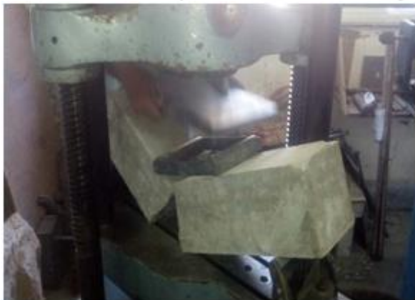
Figure 2: Flexure Beam Failure (Regular beam without any reinforcement)
