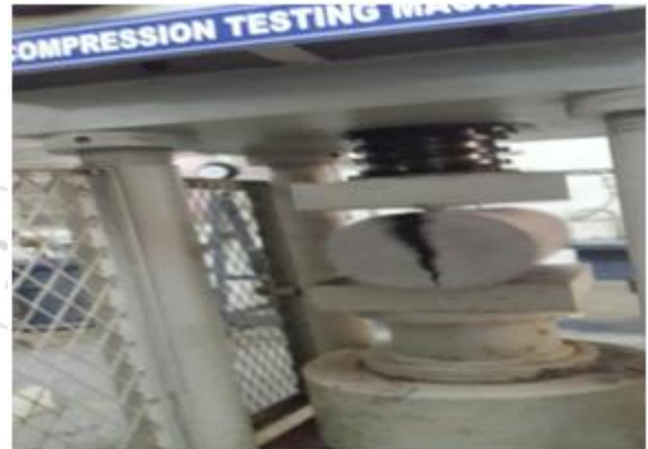
Figure 4: Loading in Progress of cylinder
