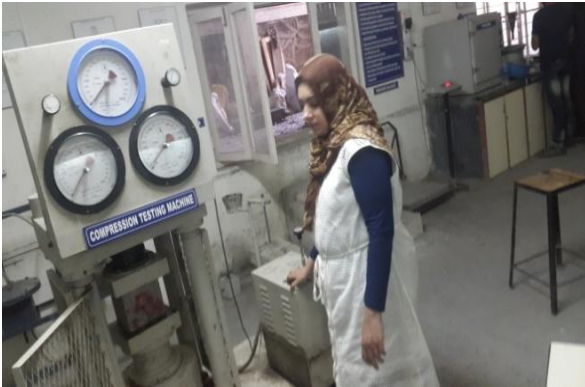
Figure 1: Cube Testing on a Compression Testing Machine
