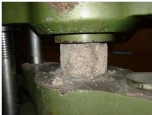
Figure 2: Cubes tested for its compressive strength in UTM
