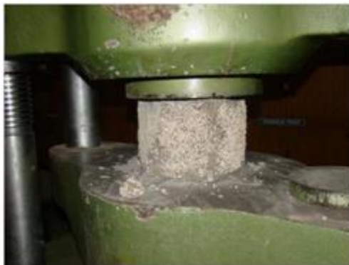
Figure 2: Cubes tested for its compressive strength in UTM
