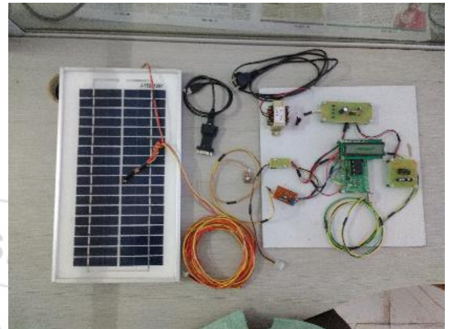
Figure (e): basic solar irradiance sensor implementation
