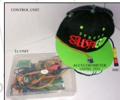
Figure 5: Real Hardware Image of Control Unit
