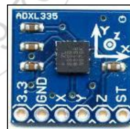
Figure 12: Accelerometer (ADXL335) Device
