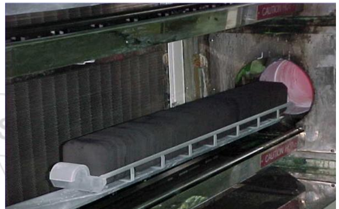
Figure 3: Solar cells placed in Diffusion Furnace
