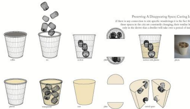
Figure 2: Ice casting forming
