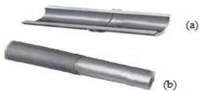
Figure 15: Cut-section of friction welded AA1100 alloy and 316 stainless steel (a) weld joint with flash removed (b).
