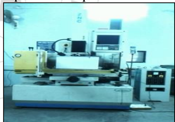
Figure 2: Powder mixed Electric discharge machining (PMEDM).
