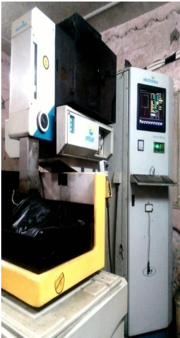
Figure2: CNC WIRE EDM Setup for machining
