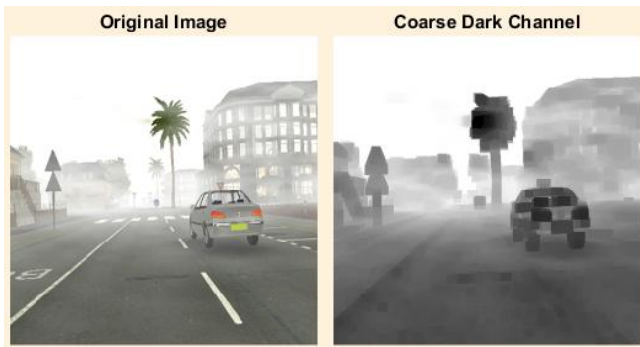
Figure 2: Dark channel haze free images (a) Haze free images (b) corresponding dark channel
