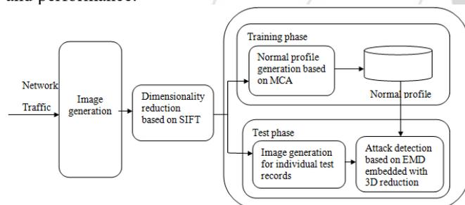
Figure 1: Denial of service attack detection system
