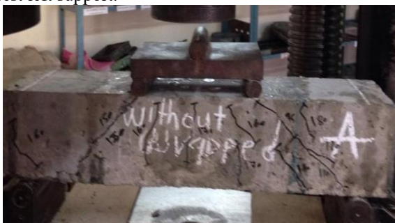
Figure 8: Crack pattern of Control Beam-A (without wrapped)
