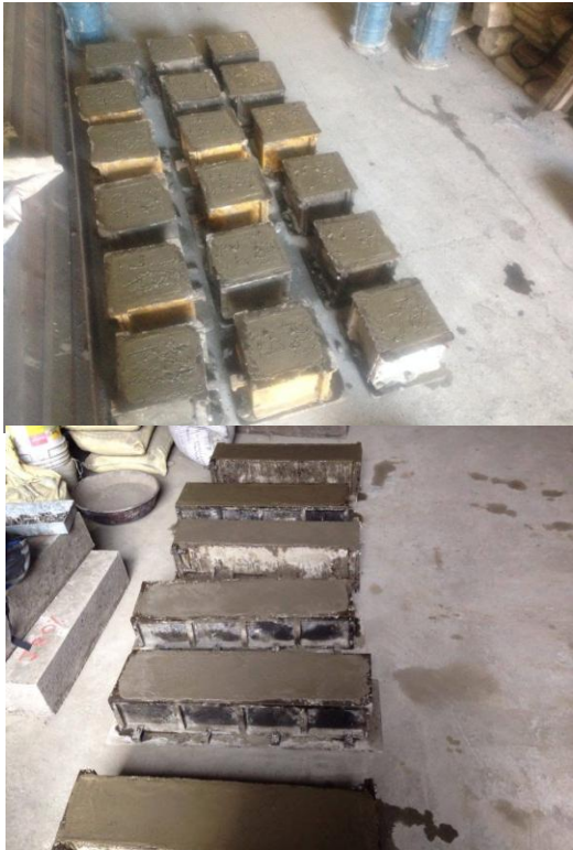
Figure 4: Details of Castings Cubes and Beams
