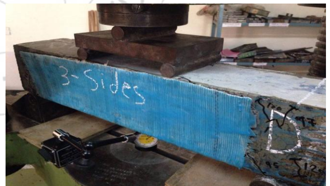
Figure 10: Crack pattern of strengthened Beam-D
