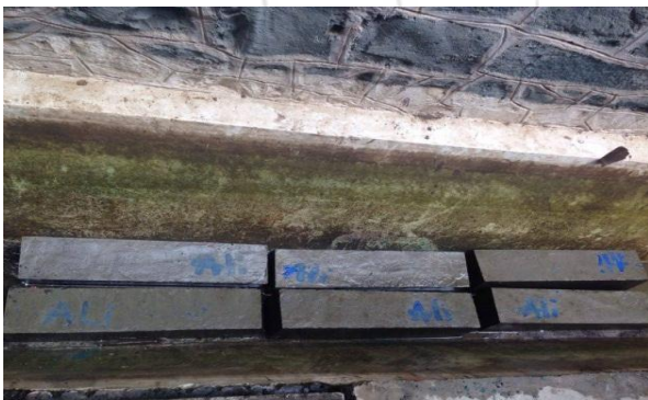
Figure 5: Curing the Specimens in Water for 28 Days
