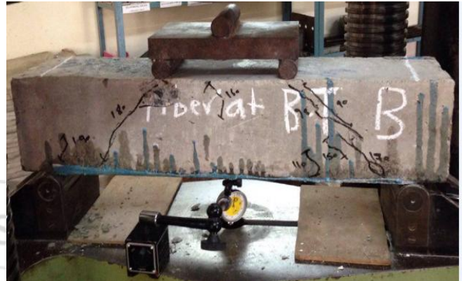
Figure 9: Crack pattern of strengthened Beam-B
