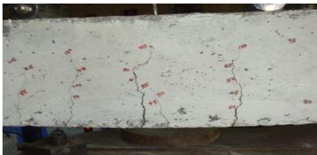
Figure 7: Flexural failure in control beam
