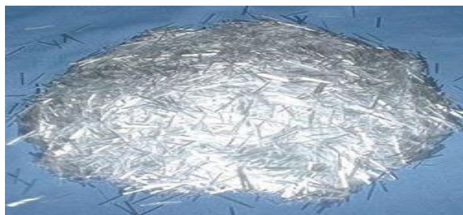
Figure 1: Glass fibres 12 mm long
