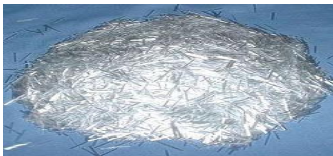
Figure 1: Glass fibres 12 mm long
