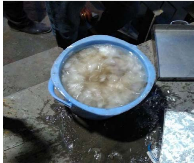
Figure 7: Glass fibre forming mesh when added to water
