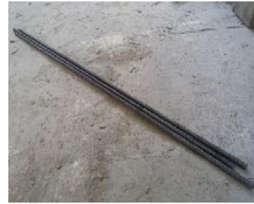
Figure 3: Steel deformed bars
