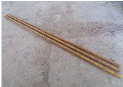
Figure 2: Sand coated GFRP bars
