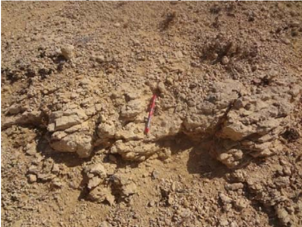
Figure 1(A): A photograph of fossiliferous limestone used for cement manufacturing in Kachchh, Gujarat
