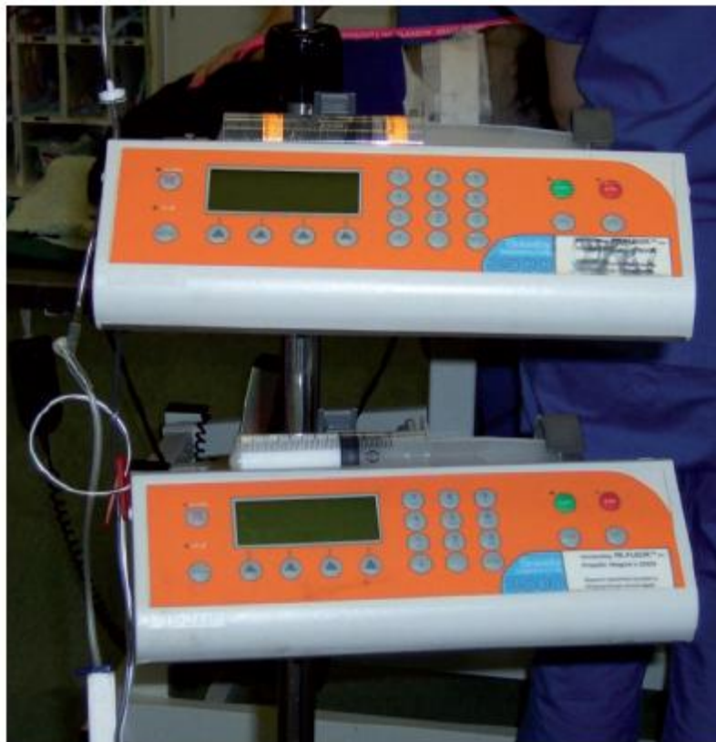
Figure 4: Two syringe drivers set in parallel during anaesthesia of dog. One infuses an analgesic (eg remifentanyl) while the other is a target-controlled infusion system to provide anaesthesia using propofol
