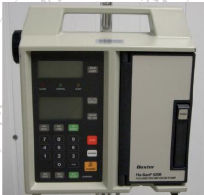
Figure 2: Volumetric Infusion pumps can be used to administer large volume infusions more accurately
