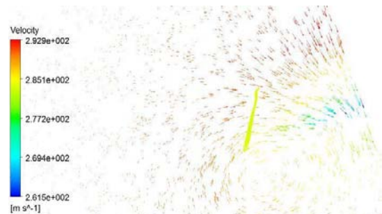
Figure 10: Velocity vectors of box wing at M = 0.73, 10° AOA and 5° cant angle
