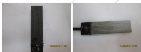
(a) Without inhibitor for 96h (b) with 10% inhibitor for 96h
