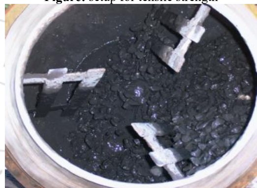
Figure: Making silica fume concrete in the laboratory
