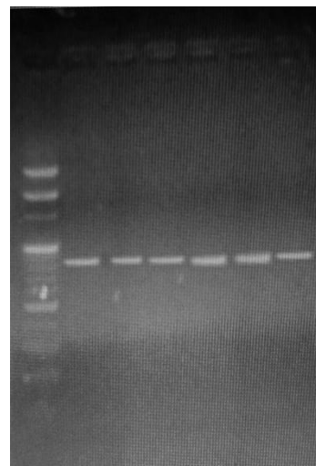
16s rDNA pcr electrophoresis image (Ladder from bottom reads 100, 200, 300, 400, 500, 600, 700, 800, 900, 1000, 1300, 1500) bp
