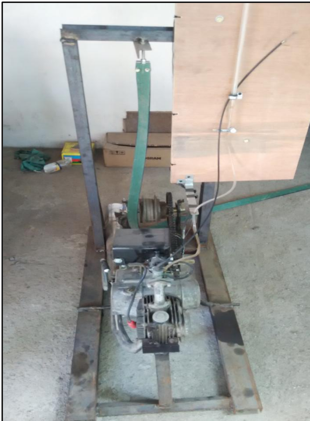
Figure 2: Actual working model of 4-stroke SI engine with methanol blend fuel
