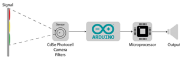
Figure 3: Block diagram of the basic visual system
