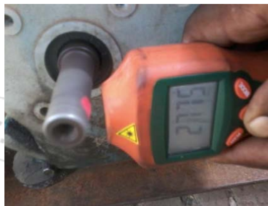
Figure 3: measuring the shaft speed of a gas driven engine using a digital tachometer
