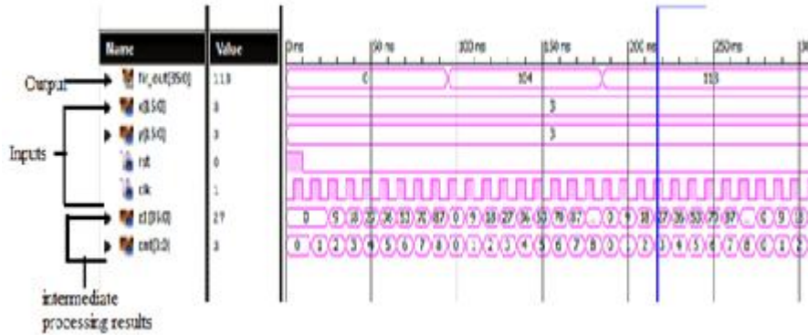
Figure 7: Simulation results for proposed 16-bit MAC Unit
