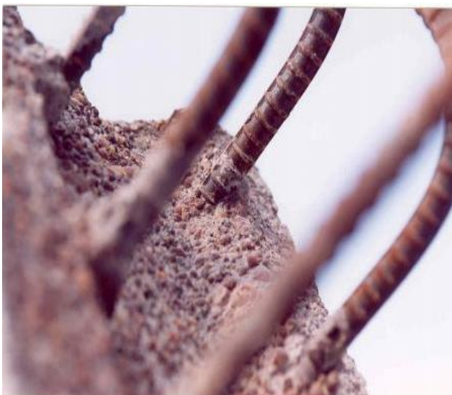
Figure 3: Steel bars and lightweight concrete bonding
